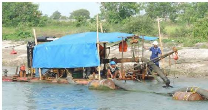
Gambar 2. 5 Suction Dredger (Adlin dkk., 2017)
