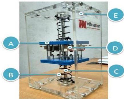
Gambar 3. 3 Cantilever piezoelectric vibration absorber (CPVA)
