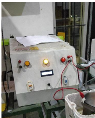
Gambar 3.2 Peralatan plasma electrolytic oxidation (PEO).
