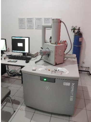
Gambar 3.4 Alat scanning electron microscope (SEM).
