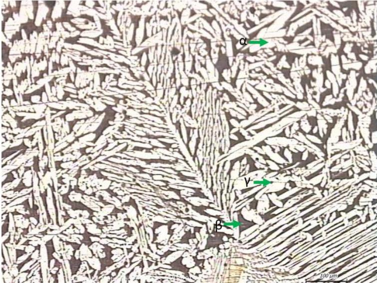
**Gambar 4. 6** Hasil Pengujian Metalografi Spesimen H850 Cu-21 Zn-5 Al *Shape memory alloys* Perbesaran 100x
