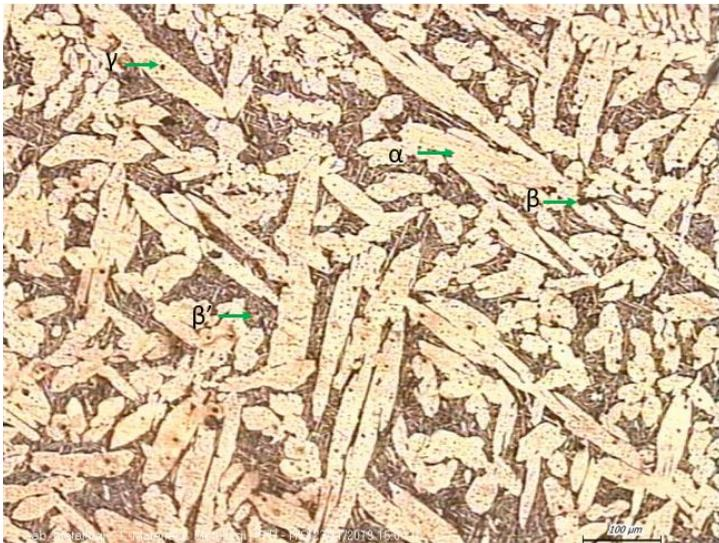
**Gambar 4. 8** Hasil Pengujian Metalografi Spesimen A550 Cu-21 Zn-5 Al *Shape memory alloys* Perbesaran 100x
