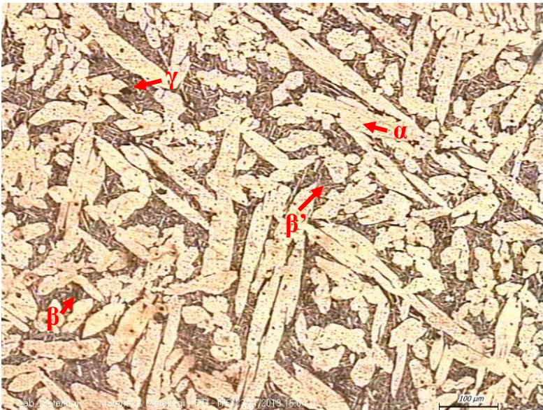
Gambar 4.8 Hasil pengujian metalografi spesimen annealing Cu-21Zn-5Al shape memory alloys perbesaran 100x
