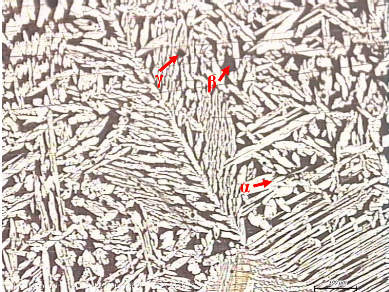
Gambar 4.6 Hasil pengujian metalografi spesimen homogenizing Cu-21Zn-5Al shape memory alloys perbesaran 100x
