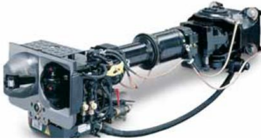
Gambar 2. 3 Coupler Scharfenberg tipe 330
