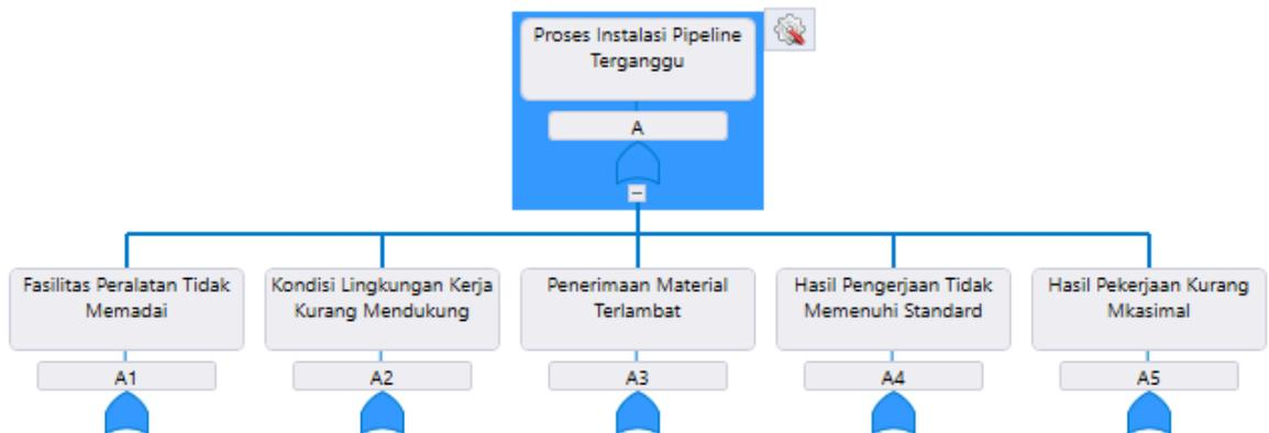
**Gambar 4.2** Diagram FTA Proses Instalasi *Pipeline* Terganggu
