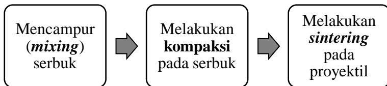
Gambar 2.2 Proses Metalurgi serbuk (Thummler, 1993)
