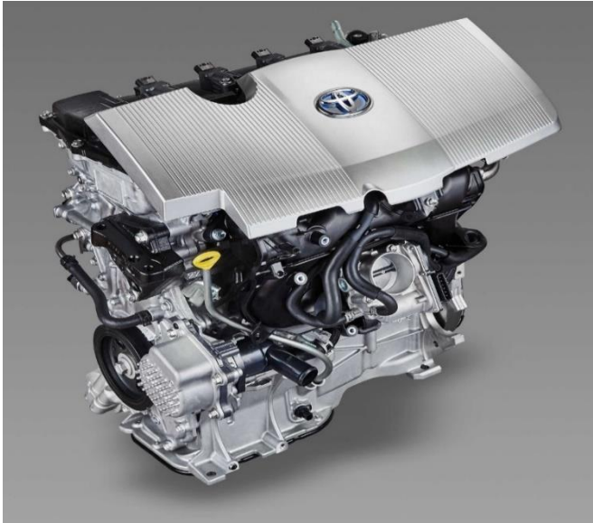
Gambar 2.12 1.8L ZR-FXE Toyota Prius internal combustion engine .
