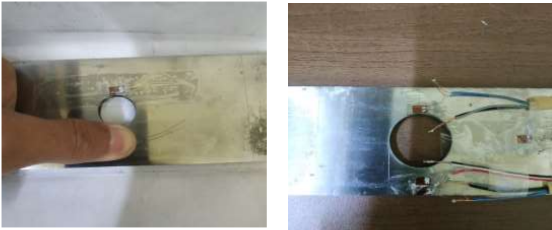
Gambar 3.25 Pemasangan sensor strain gauge
