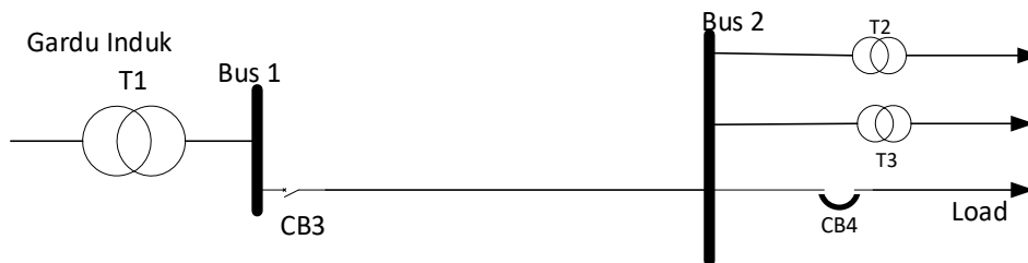
Gambar 2. 2 Sistem Distribusi Radial
