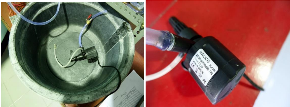
Gambar 3.2 pompa, valve, reservoir
