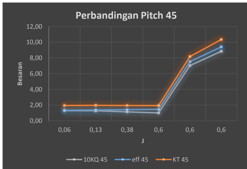
Gambar 4. 3 Kavitasasi C4-40 Pitch Angle 45°
