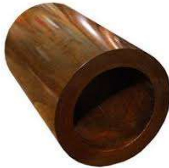
Gambar 2. 4 Bearing sterntube kayu poghout
