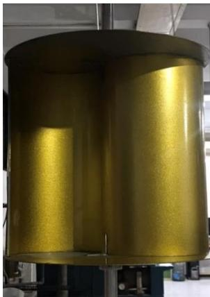
Gambar 3. 5 Turbin Savonius
