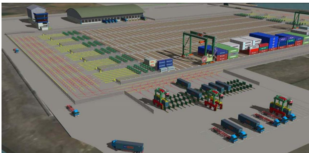
Gambar 2.4 Landside Transfer Area
