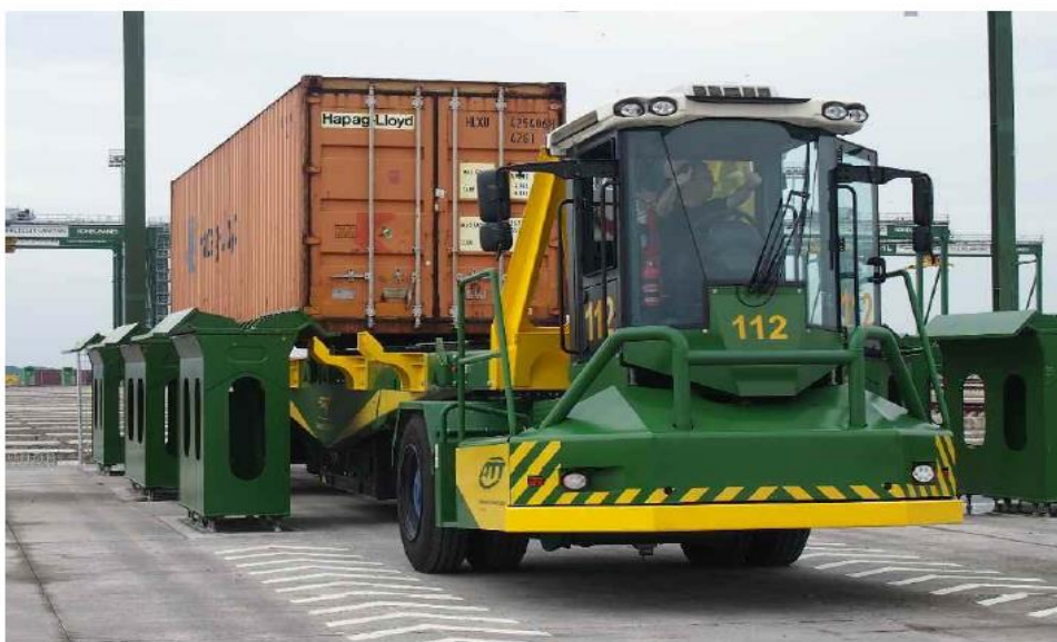
Gambar 2.5 Combine Terminal Truck
