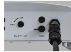
▲ Figure 4.16 Connect the Terminal Connector to the Inverter
