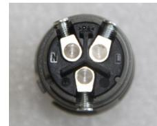
▲ Figure 4.11 AC Grid Terminal Connector Inside
