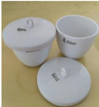
**Gambar 3.10** *Crucible furnace*
