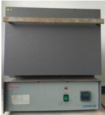
**Gambar 3.11** *Muffle furnace*
