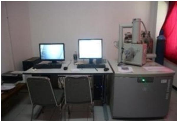
**Gambar 3.13** Alat uji SEM-EDX FEI tipe Inspect S-50
