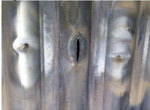
**Gambar 2.5** *Hydrogen damage pada tube boiler (Dooley and McNaughton, 1995)*
