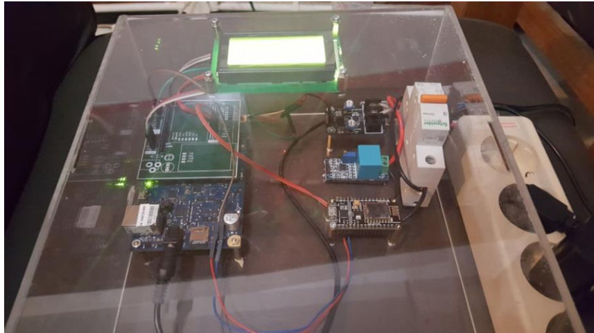
Gambar 3.12 Desain hardware Smart meter
