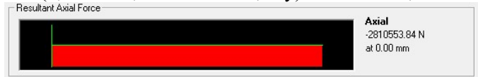
Gambar 4.46 Gaya Axial Terhadap Kombinasi (1.2DL + 1.0LL + 1.0Ey + 0.3Ex) P_u (1,2DL + 1,0 LL + 0,3Ex + Ey) = -2810553,84 \text{ N}
