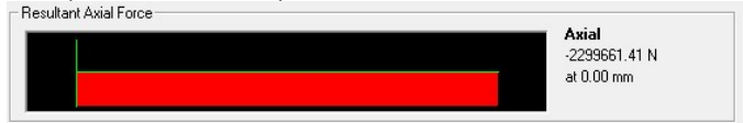
Gambar 4.45 Gaya Axial Terhadap Kombinasi (1.2DL + 1.0LL + 1.0Ex + 0.3Ey) P_u (1,2DL + 1,0 LL + Ex + 0,3Ey) = -2299661,41 \text{ N}
