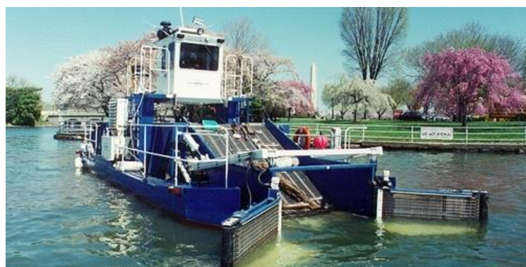
Gambar II.5 Trash Skimmer Boat saat Beroperasi (Sumber: http://www.mudcatdredge.com/trash-skimmer-vessels , 2019)
