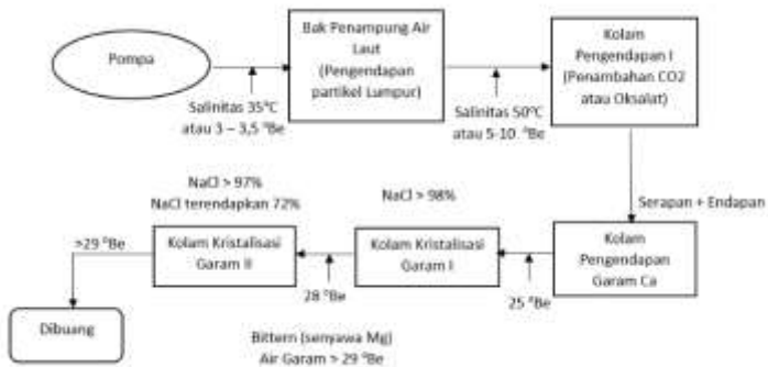
Gambar III.4 Diagram proses penguapan air laut ( solar evaporation )
