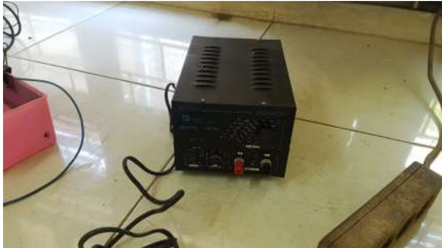
Gambar 3.16 DC Power Supply
