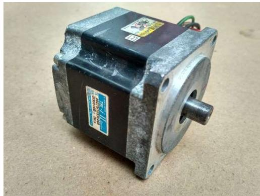
Gambar 2.13 Generator Tamagawa TBL-i II Series TS4607N1033E200
