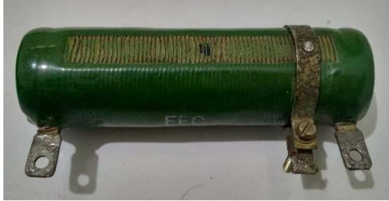
Gambar 3.23 Wirewound Resistor
