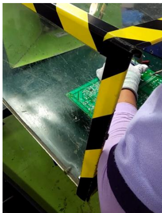
Gambar 4.10 Proses Inspection & Touch Up
