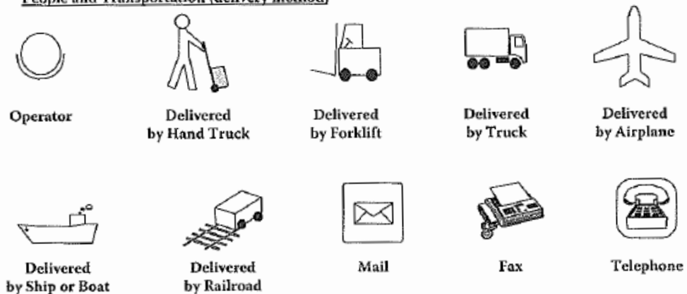
Gambar 2.1 Simbol Dasar Value Stream Mapping Sumber: Nash dan Poling (2008)
