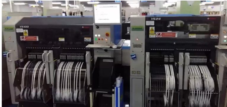
Gambar 4.5 Proses SMT ( Mounter )
