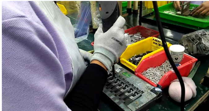
Gambar 4.7 Proses Forming Komponen L101 Ferrite Bead
