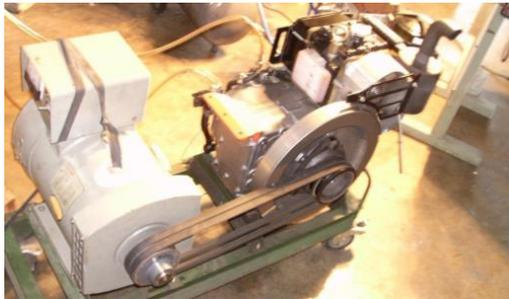
**Gambar 3.3** Satu set engine diesel (Yanmar) – generator (Noqiwa)
