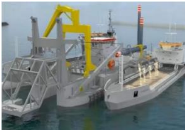
Gambar 7 7 Proses Pengisian Barge (Barge Loading)
