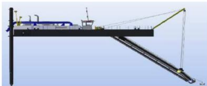
Gambar 4 8 Contoh Kapal CSD500 Damen (Sumber: brosur Damen Dredging Equipment)
