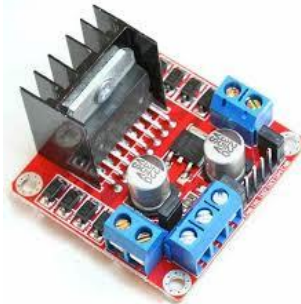
Gambar 2.4. Modul driver L 298
