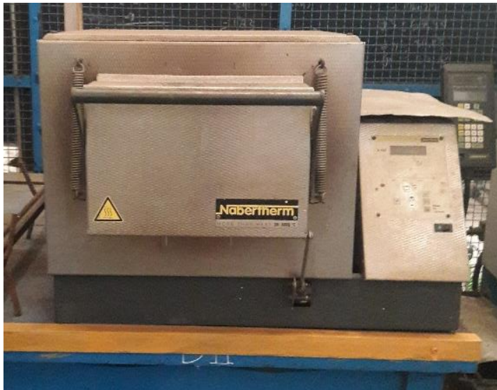
Gambar 3.4 electric resistance furnace in heat treatment workshop Departemen Teknik Mesin FTI-ITS
