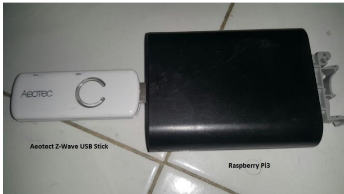
Gambar 3. 1 Raspberry Pi 3 dan Aeotec Z-Wave USB Stick
