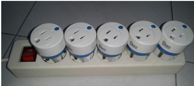
Gambar 3. 5 Z-Wave Smart Plug Neo Coolcam
