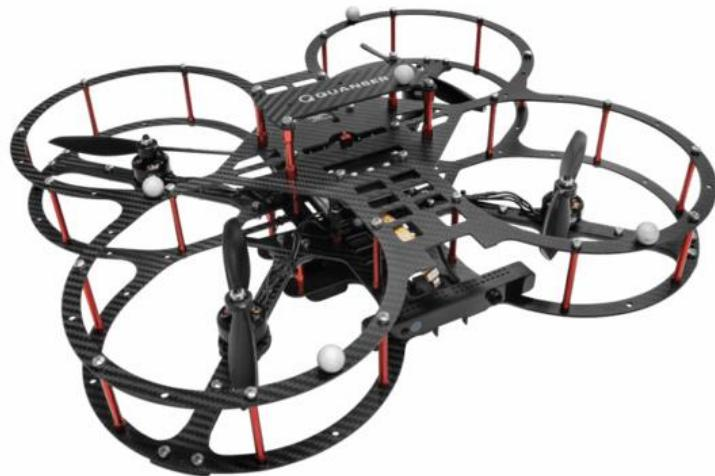
Gambar 3.1 Quadcopter Quanser Qdrone
