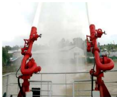
Gambar 8. Fire Monitor Sumber: Nedved Jiang, 2007
