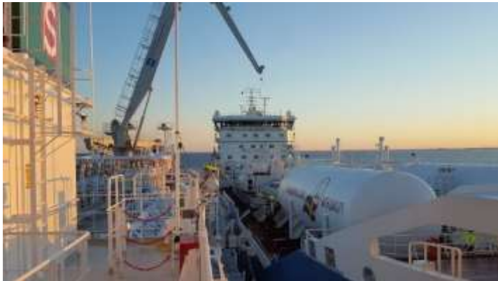
Figure 2. 5 The Bunkering of LNG Cargo (Source: marine-executive.com)
