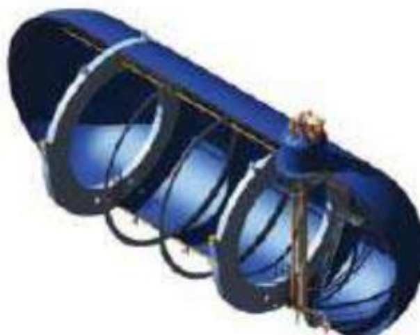
Gambar 2.10 LNG double skinned tanks Sumber : ABS, 2011, LNG Powered Vessels and the ABS Guide for the propulsion and auxiliary Systems for Gas fueled Ships
