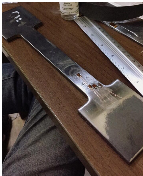
Gambar 3.33 Pemasangan sensor strain gauge
