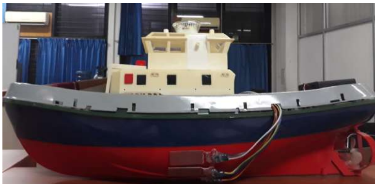
Figure 4.14 Water Level Sensor Installation
