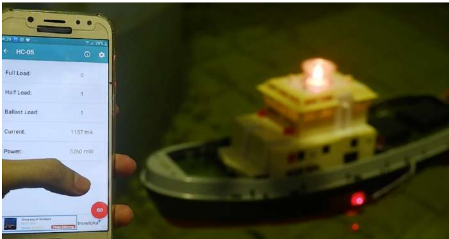
Figure 4.21 Monitoring Simulation at Half Load Condition
