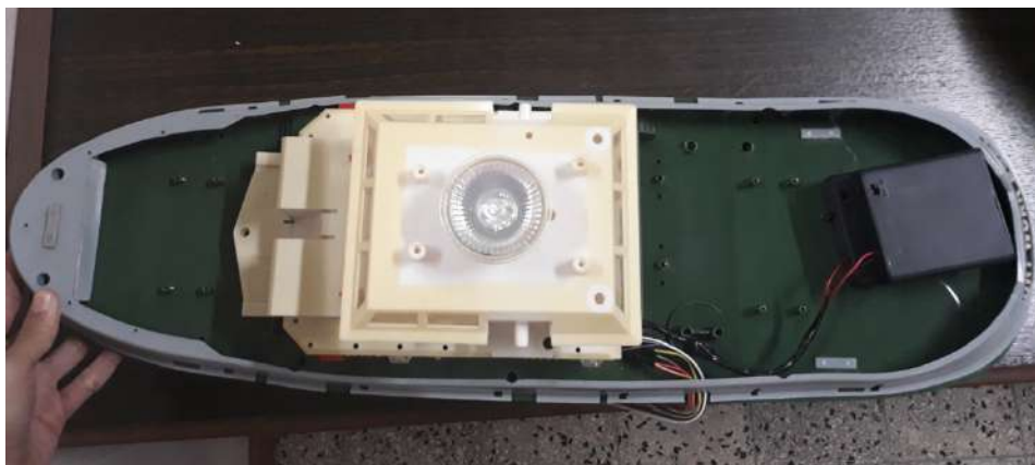
Figure 4.15 LED and Power Supply Installation
