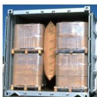
Figure 7.9 Gap filled with a central dunnage bag
