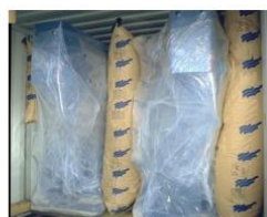
Figure 7.10 Irregular shaped packages blocked with dunnage bags
