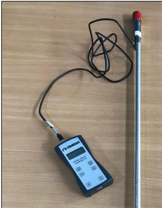
Gambar 3. 9 Anemometer Omega HHF141
