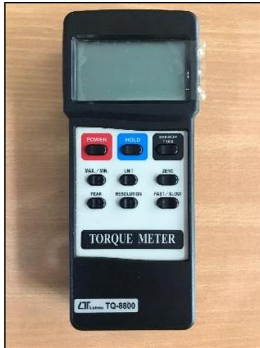
Gambar 3. 12 *Torque meter* Lutron model TQ-8800
