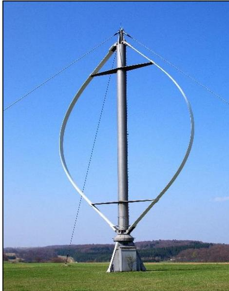
Gambar 2.2 Turbin Darrieus (Sumber : <https://en.wind-turbine-models.com/turbines/93-dornier-darrieus-55>)
