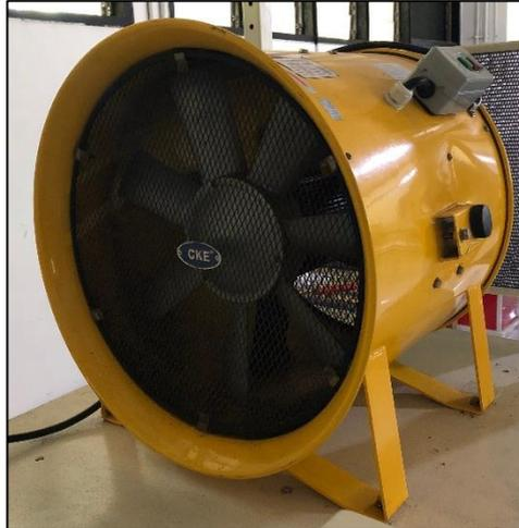
Gambar 3. 3 *Axial Fan* CKESPV-18
