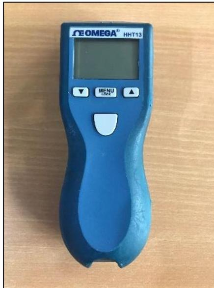
Gambar 3. 10 Tachometer OMEGA HHT12
