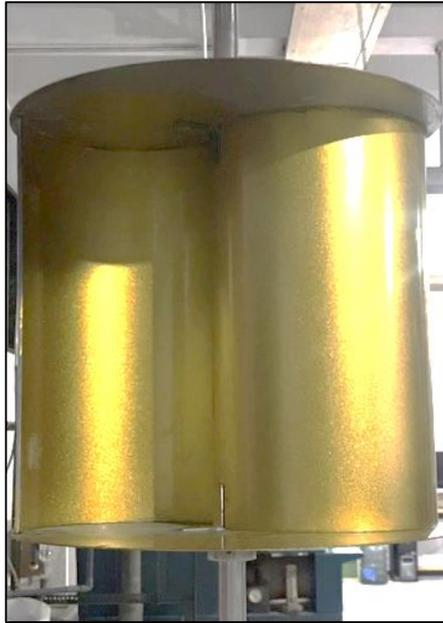
Gambar 3. 6 Turbin Angin Savonius
