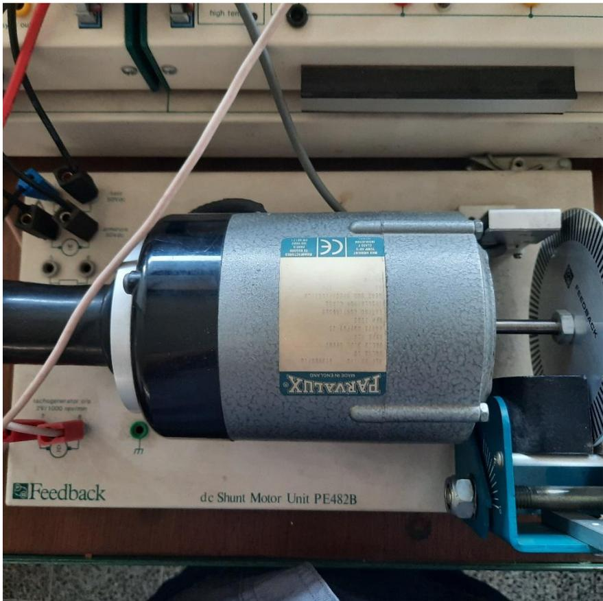
Gambar 3. 2 Motor DC Shunt
