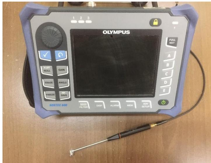
Gambar 3.10 Mesin Eddy Current Testing
