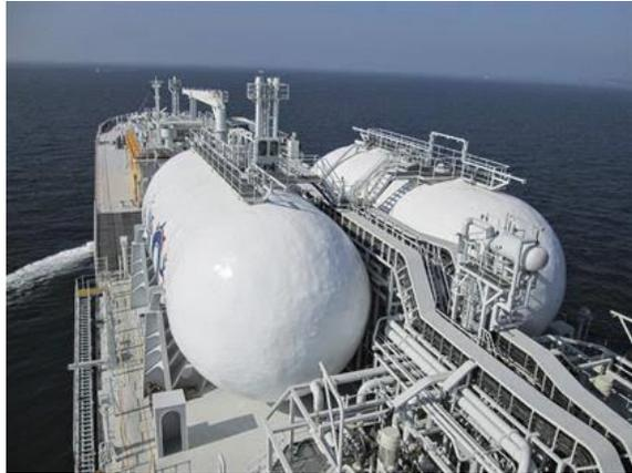
Gambar 2.16 LNG Type C Tank
