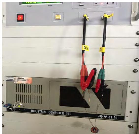
Gambar 4.6 Mesin uji *hysteresis graph meter*
