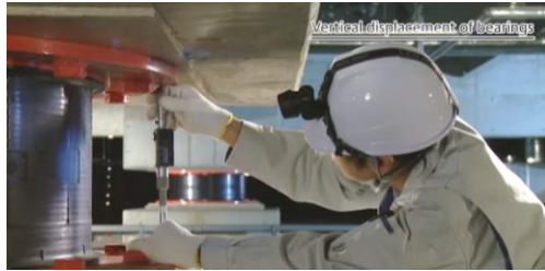
Gambar 10. 20 Pengecekan perpindahan vertikal (Bridgestone, 2013)
