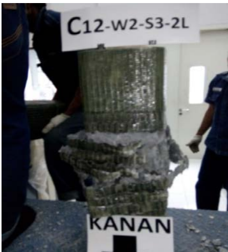
Gambar A18 Pengujian specimen kolom beton E-GFRP C12-W2-S3-2L
