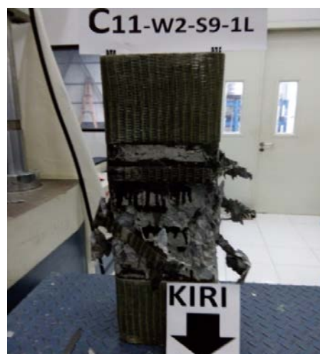
Gambar A17 Pengujian specimen kolom beton E-GFRP C11-W2—S9-1L
