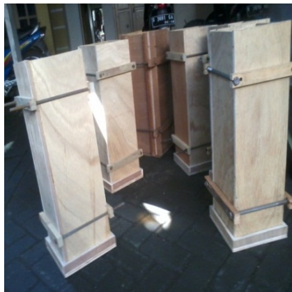
(c) Bekisting benda uji kolom
