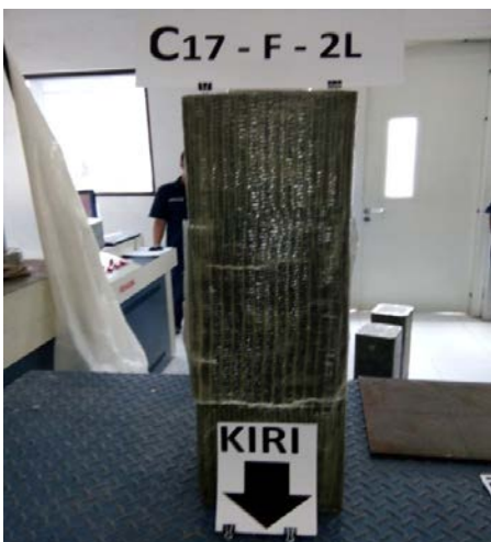
Gambar A22 Pengujian specimen kolom beton E-GFRP C17-F-2L
