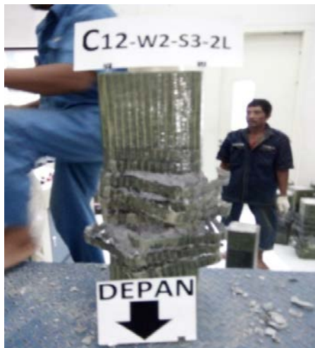
Gambar A18 Pengujian specimen kolom beton E-GFRP C12-W2-S3-2L
