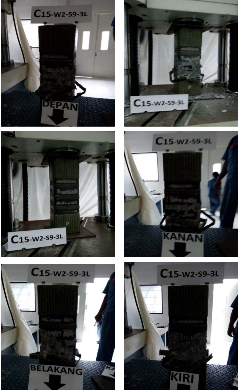
Gambar A20 Pengujian specimen kolom beton E-GFRP C15-W2-S9-3L
