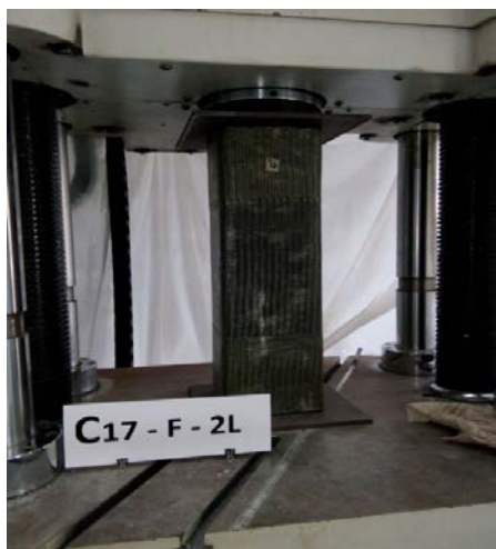
Gambar A22 Pengujian specimen kolom beton E-GFRP C17-F-2L
