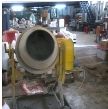
(b) Concrete mixer kapasitas 0.05m^3
