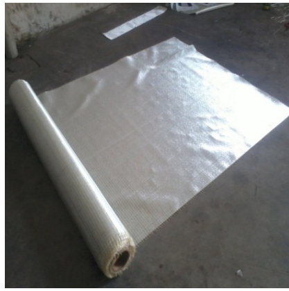
(b) E-GFRP sheet (TYFO SH25)
