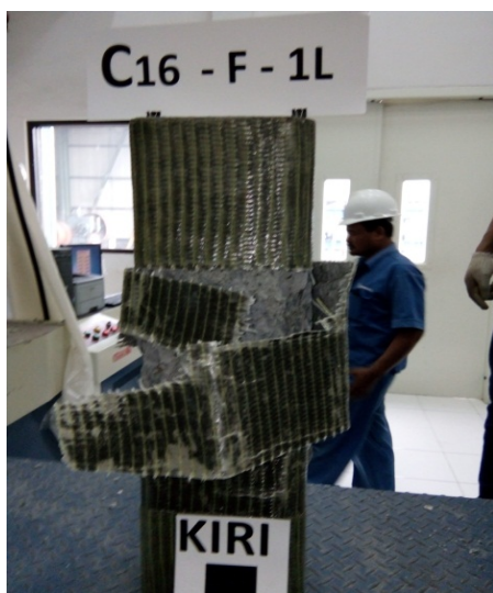
Gambar A21 Pengujian specimen kolom beton E-GFRP C16-F-1L
