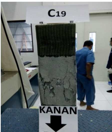
Gambar A24 Pengujian specimen kolom beton E-GFRP C19
