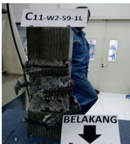
Gambar A17 Pengujian specimen kolom beton E-GFRP C11-W2—S9-1L
