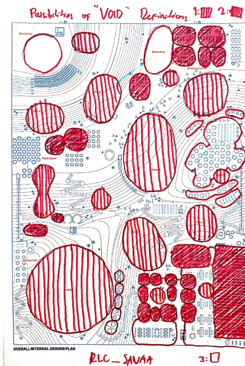
Figure 3.7. Precedent Study: Possibilities of solid-void definitions in Rolex Learning Centre by SANAA
