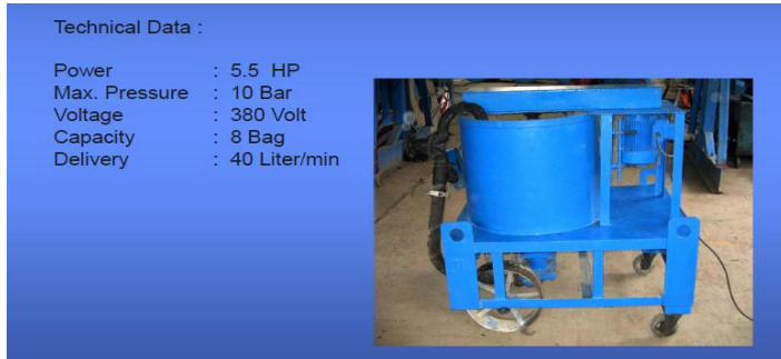
Gambar 4. 31GROUT Pump
