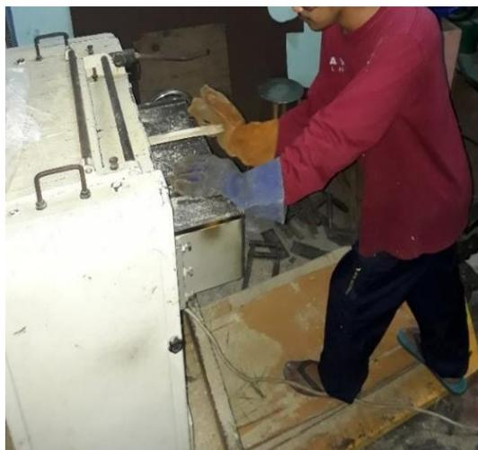
Gambar 4. 9 Proses Penipisan Bambu
