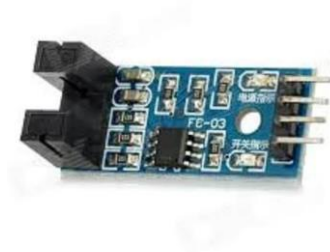
Gambar 2.15 Modul sensor FC-03 (“Motor Encoder RPM Speed Counter Interrupter Sensor Module FC-03 | QQ Online Trading,” 2019)
