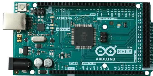
Gambar 2.16 Arduino Mega 2560 (“Arduino - ArduinoMega2560,” 2019)
