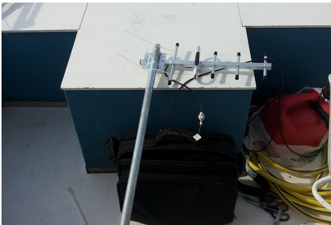
Gambar 2.16: End Node menggunakan Antenna Digital Outdoor di Laut Tyrrhenian, Italia [13]
